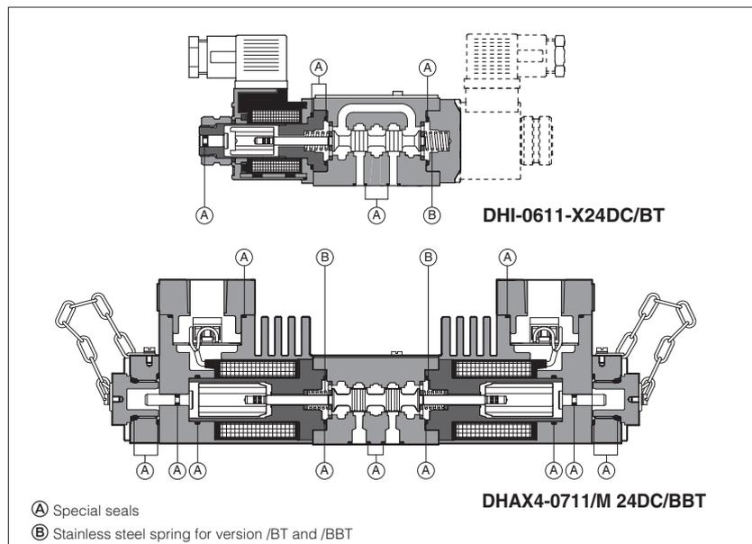
Standard and special components equipped with specific seals for applications at high / low temperatures or with aviation hydraulic fluids.
