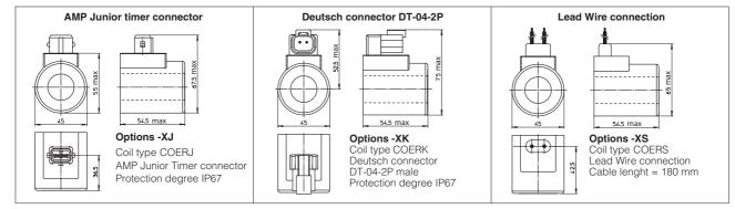
Note: The above coils are available only for voltage supply 12, 14, 24 and 28 Vpc. For the characteristics refer to standard coils features - see sect. (5)
