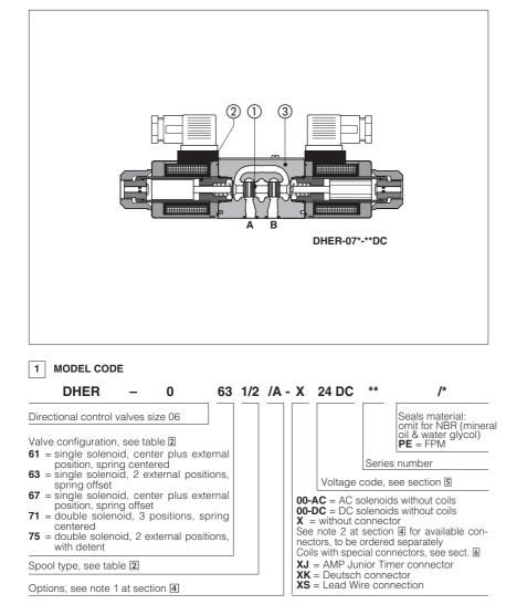
Spool type, direct operated solenoid valves equipped with threaded type, high performance solenoids certified according the North American standard **cUR**us
