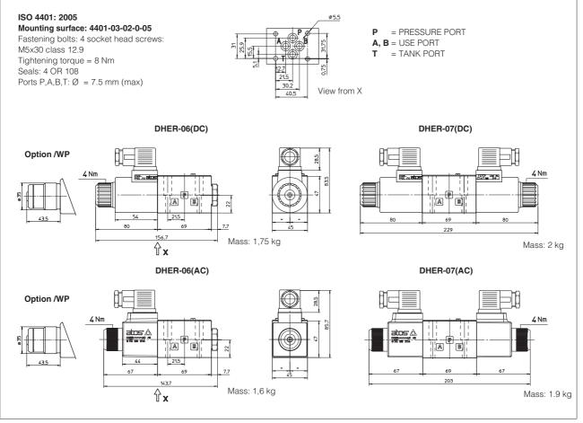
Overall dimensions refer to valves with connectors type 666
