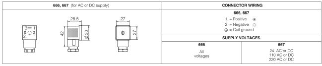
12 COILS WITH SPECIAL CONNECTORS only for voltage supply 12, 14, 24, 28 VDC
