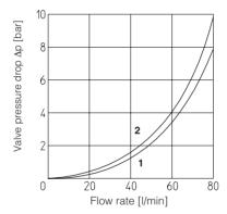
Valve pressure drop - NC version  $\mathbf{3}$ = flow B  $\rightarrow$  A energized
