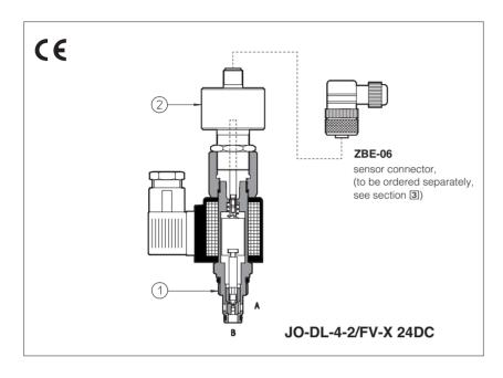
JO-DL are leak free, poppet type solenoid cartridges in screw-in execution normally used to cut off the hydraulic power supply line. They are available in normally closed NC, or normally open one NO configurations.
