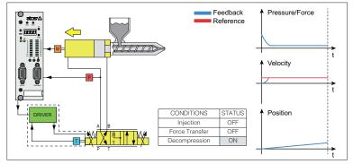
3.4 Back Pressure - Pressure closed loop control with max velocity limitation
