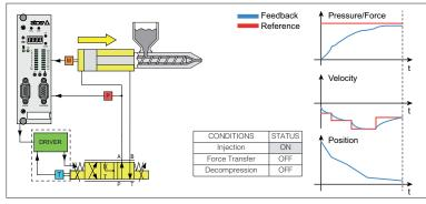
3.2 Pack and Hold - Pressure closed loop control with max velocity limitation
