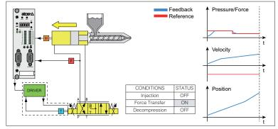
3.5 Post-Decompression - Velocity open loop control
