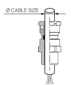
Cable glands for use with non-armoured plastic insulated cables
