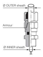
Cable glands for use with single wire armour 'W', wire braid 'X', steel tape armour 'Z', plastic insulated cables.
