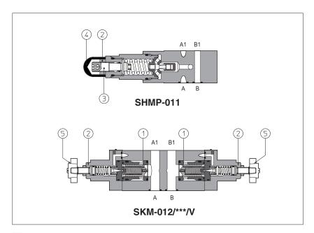
SHMP are direct operated pressure relief valves, size 06.
