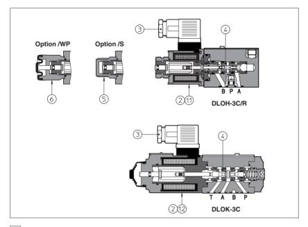
DLOH and DLOK are poppet type, two or three way, two position direct operated solenoid valves, designed to operate in oil hydraulic systems with leak free require-
