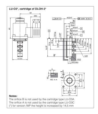
These cartriges can be installed in the manifolds
