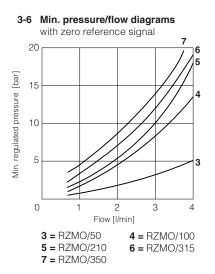
Note: the presence of counter pressure at port T can affect the pressure regulation and the minimum pressure
