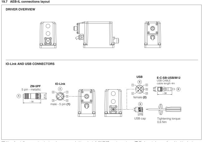
(1) Use of metallic connectors is strongly recommended in order to fulfill EMC requirements
