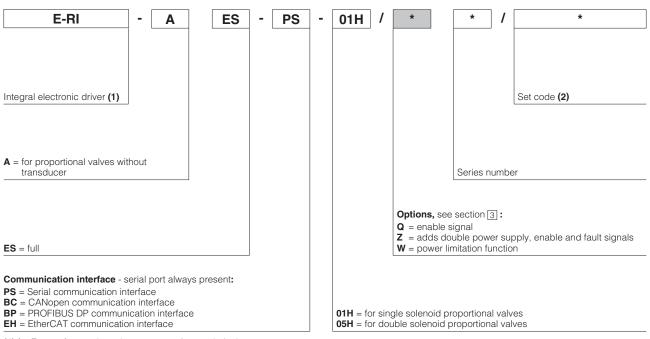
(1) for Ex-proof execution, please contact Atos technical support(2) set code identifies the corrispondance between the integral driver and the relevant valve; it is assigned by Atos when the driver is ordered as spare part
