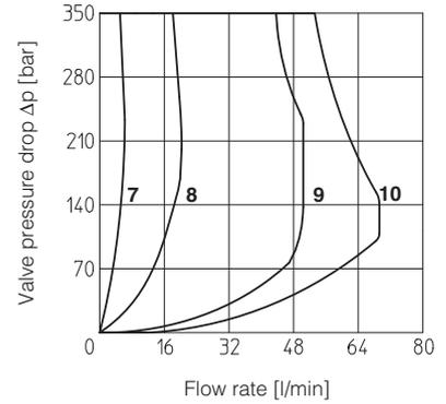
**8 DIAGRAMS FOR SDKZE** (based on mineral oil ISO VG 46 at 50 °C)
