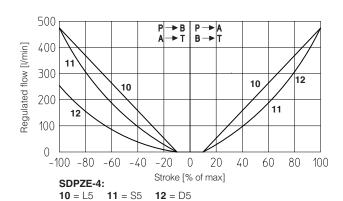
**Note**: Hydraulic configuration vs. reference signal for configuration 71 and 73 (standard and option /B)
