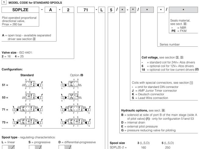
(1) In standard configuration the solenoid (config. 51 and 53) is at side A of the main stage (side B of pilot valve)
