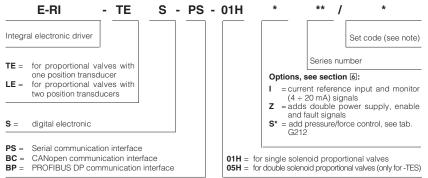
Note: The set code identifies the correspondance between the digital integral driver and the relevant valve; it is assigned by Atos when the driver is ordered as a spare part
