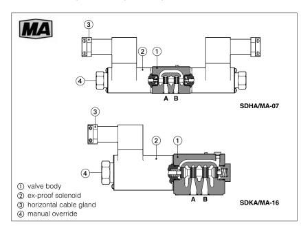
Directional and pilot operated pressure relief valves equipped with explosion-proof solenoids certified according to **MA** Chinese mining certification, protection mode:
