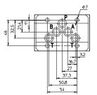
P = PRESSURE PORT A, B = USE PORT T = TANK PORT
