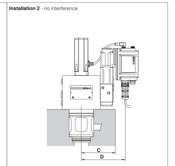
${\bf C}={\bf Max}$  manifold dimension to avoid interference with the main connector, see below table
