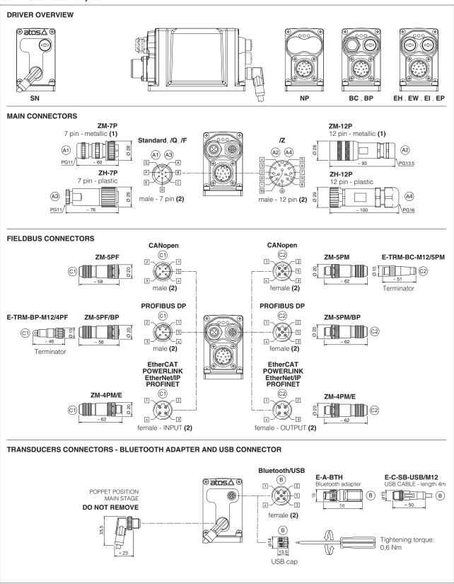
(1) Use of metallic connectors is strongly recommended in order to fulfill EMC requirements
