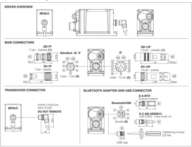
(1) Use of metallic connectors is strongly recommended in order to fulfill EMC requirements
