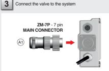
NOTE: the use of above metallic connectors is strongly recommended in order to fulfill EMC requirements
