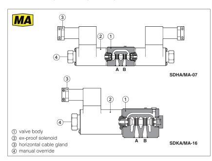
Directional and pilot operated pressure relief valves equipped with explosion-proof solenoids certified according to **MA** Chinese mining certification, protection mode:
