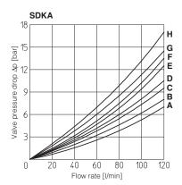
7 OPERATING LIMITS For a correct valve operation do not exceed the max recommended flow rates (I/min) shown in the below tables
