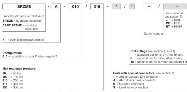
(1) select valve's coil voltage /18 in case of electronic drivers not supplied by Atos, with power supply 24Vpc and with max current limited to 1A.
