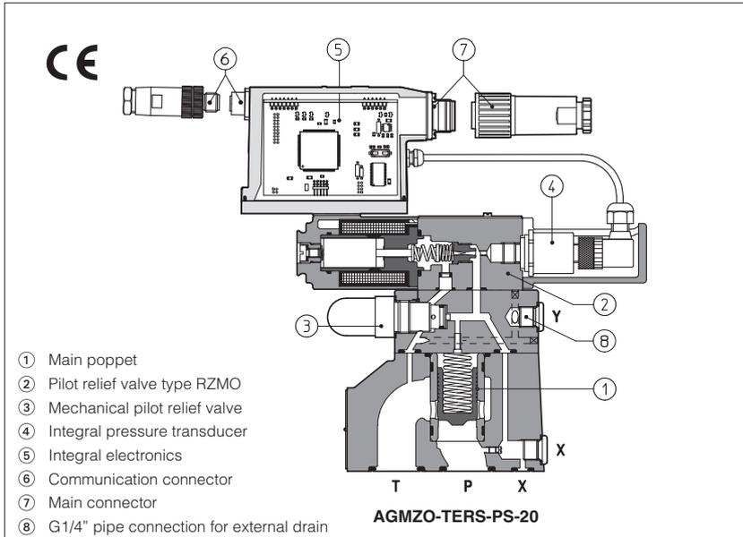
AGMZO are two stage poppet type proportional pressure relief valves, with integral or remote pressure transducer, which provide pressure regulation proportional to electronic reference signal.
