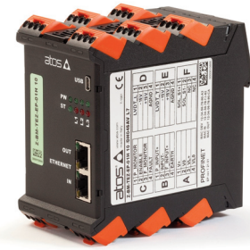
DIN-rail axis card with driver function
