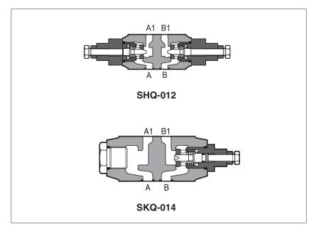
**SHQ** and **SKQ** are flow throttling valves, not compensated, and with check valve to allow free reverse flow.
