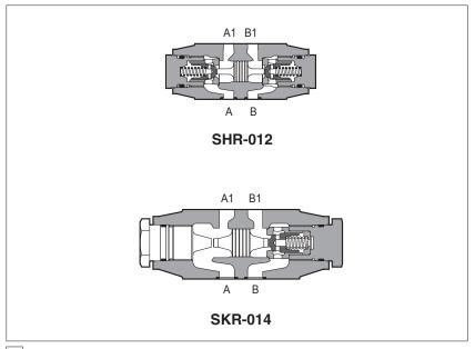
**SHR, SKR** are check valves available in direct or pilot operated models.
