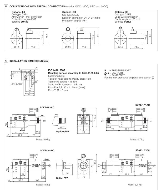
① Standard manual override PIN. The manual override operation can be possible only if the pressure at T ports is lower than 50 bar
