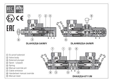
New line of directional solenoid valves and pressure relief valves in stainless steel execution for corrosive environments. Ex-proof Stainless steel solenoids ①, with **ATEX, IECEx, EAC Multicertification** or **cULus** North American certification, for hazardous areas - see section ⑤, ⑥.
