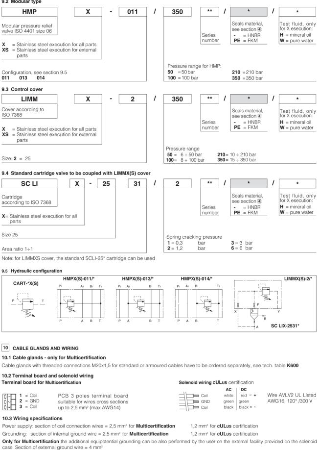
For Multicertification the cable must be suitable for the working temperature as specified in the "safety instructions" delivered with the first supply of the products.
