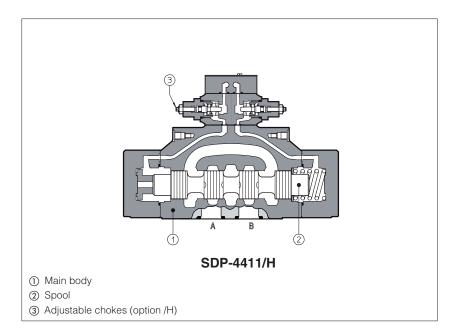
Spool type hydraulic operated directional valves in three or four way, two or three position, designed to operate in oil hydraulic systems.
