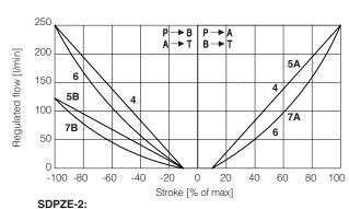
**5A** = DL5 (P $\rightarrow$ A, A $\rightarrow$ T) **7A** = D5 (P $\rightarrow$ A, A $\rightarrow$ T) **4** = L5 **5B** = DL5 (P  $\rightarrow$  B, B  $\rightarrow$  T) **7B** = D5 (P  $\rightarrow$  B, B  $\rightarrow$  T)
