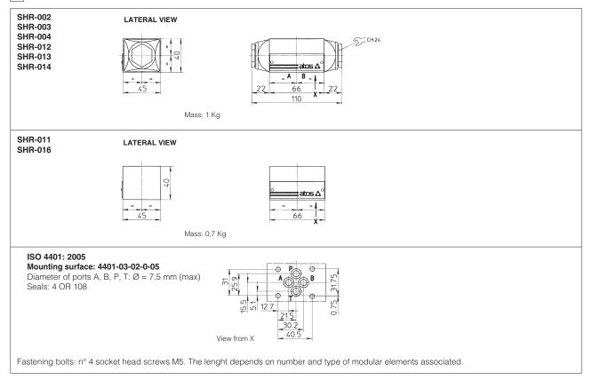
7 INSTALLATION DIMENSIONS OF SKR-0 VALVES [mm]
