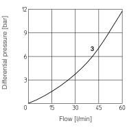
5 DIAGRAMS OF SKR-0 based on mineral oil ISO VG 46 at 50°C
