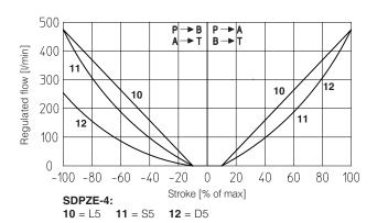
**Note**: Hydraulic configuration vs. reference signal for configuration 71 and 73 (standard and option /B)
