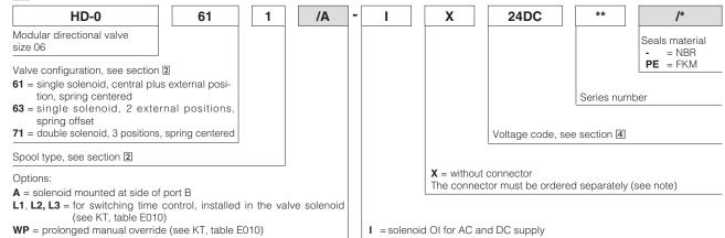
Type of electric/electronic connector DIN 43650 to be ordered separately (for overral dimensions see table K500):
