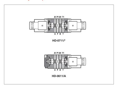
HD are spool type, direct operated solenoid valves in modular execution.
