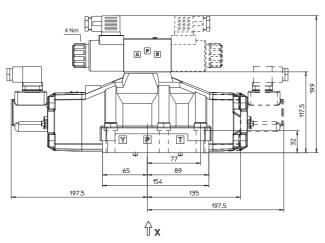
Note: for configurations 71 and 75 the switch position is on both sides of the valve
