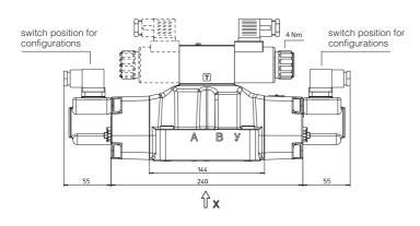
Note: for configurations 71 and 75 the switch position is on both sides of the valve
