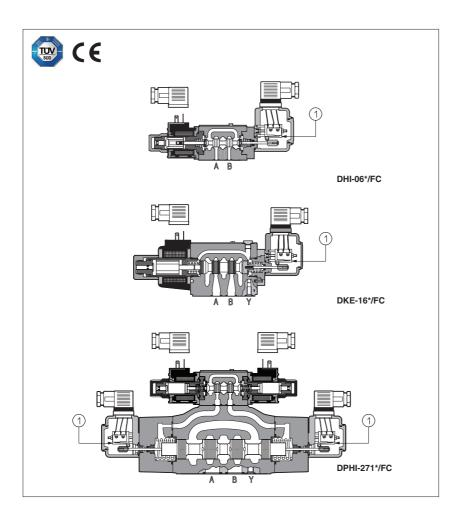
These valves are provided with **FC** mechanical microswitch ① for the spool position monitor and they are designed to fulfil the safety criteria imposed to machine manufacturers by the European Machine Directive.
