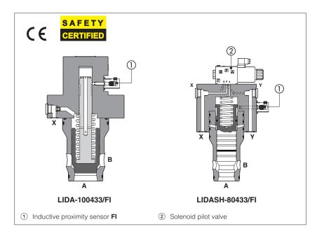
Safety cartridge valves with FI inductive proximity for poppet position monitoring, CE marked and certified by TÜV, in accordance with safety requirements of Machine Directive 2006/42/EC.
