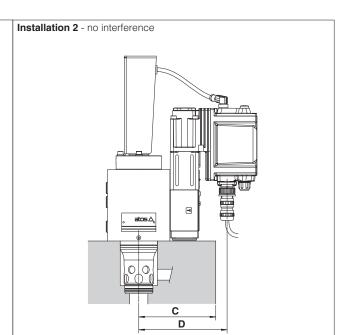
**C** = Max manifold dimension to avoid interference with the main connector, see below table
