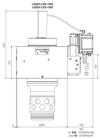
① Space to remove the 7 or 12 pin main connector. For main and communication connectors see section 11, 12
